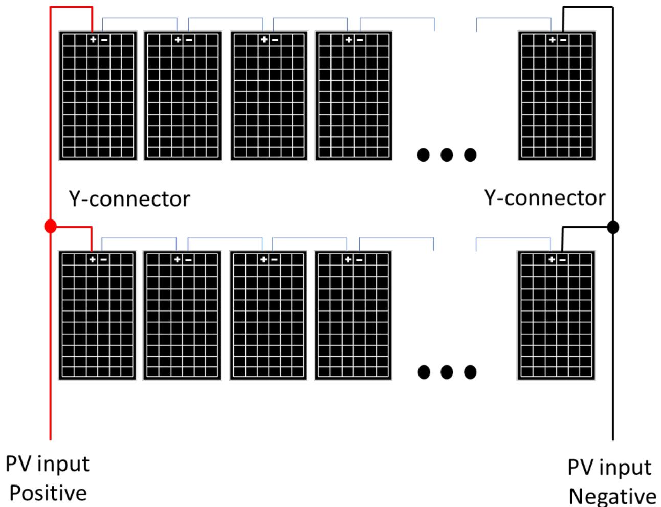
**If using Y-Connectors:** (Running two strings in parallel, totaling 20A (self-limiting) Note: separate wires can be used per string, and string minimum is usually 5 panels or 175V)
