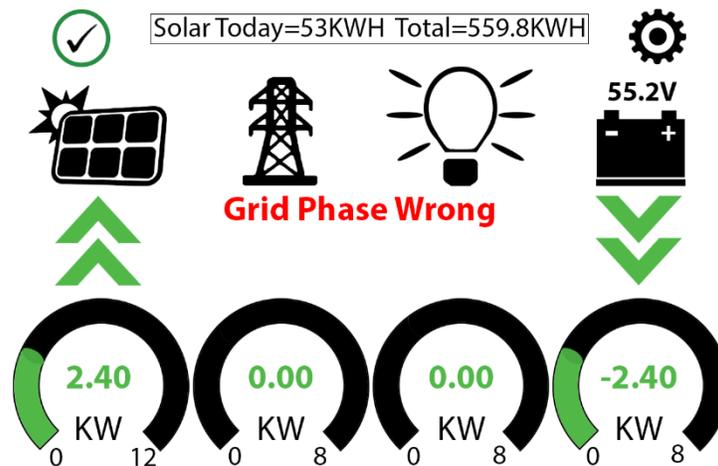
If the Sol-Ark screen shows the above error, there is a phasing issue with your wiring. This will cause overload faults (F18, F26, F34) even with the Load breaker off and **WILL cause damage if left unchecked**.
